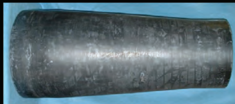
CMC combustor liner
